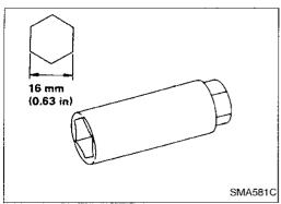
2. Remove spark plugs with spark plug wrench.
