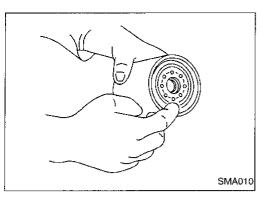
Clean oil filter mounting surface on cylinder block. Coat rubber seal of new oil filter with engine oil.
